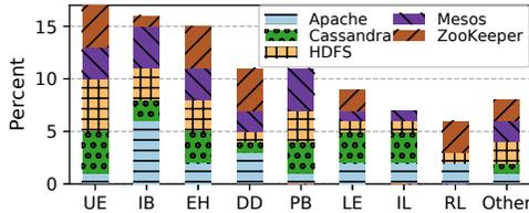
**Figure 2:** Root cause distribution. *UE*: uncaught error; *IB*: indefinite blocking; *EH*: buggy error handling; *DD*: deadlock; *PB*: performance bug; *LE*: logic error; *IL*: infinite loop; *RL*: resource leak.
